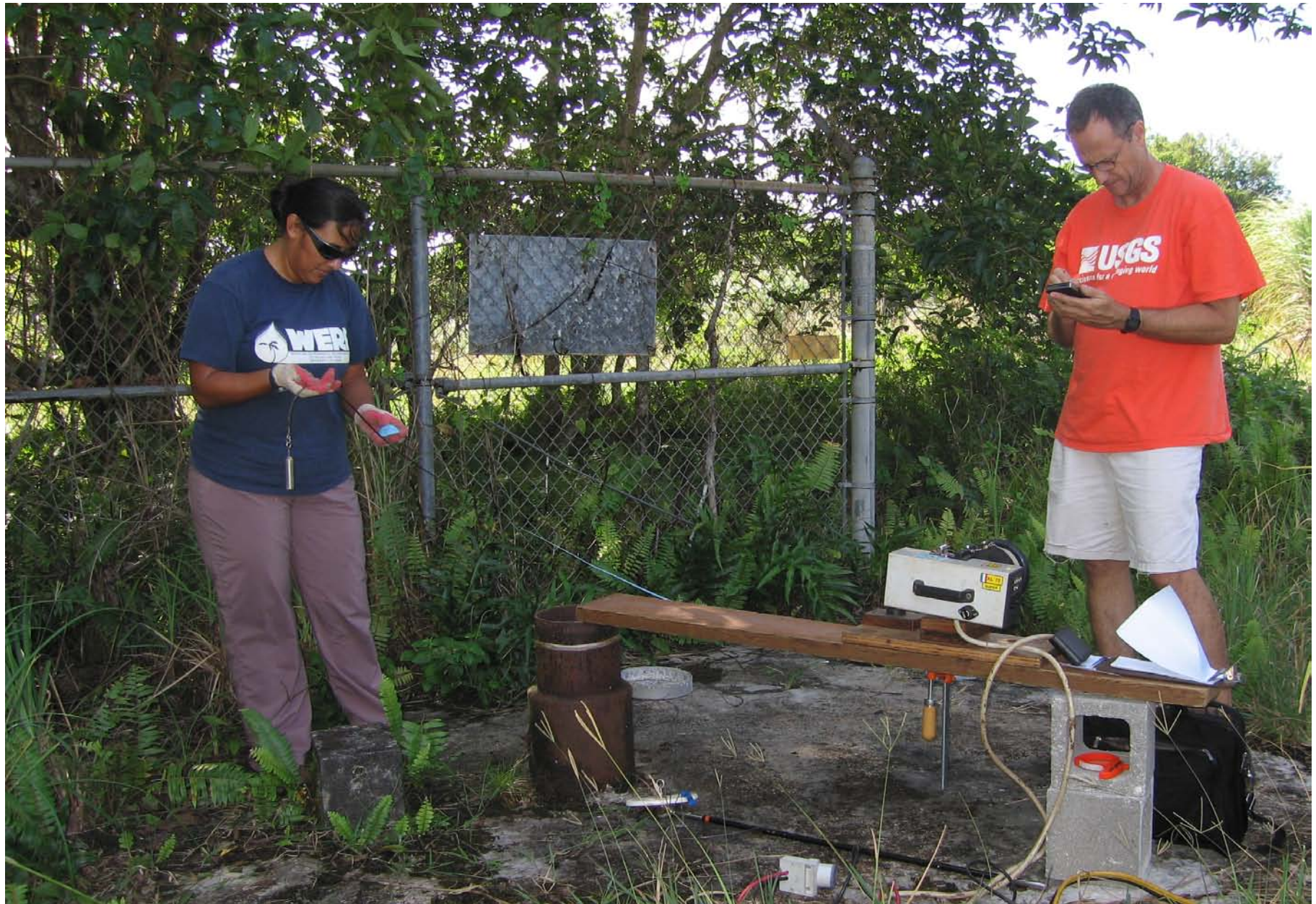
WERI Graduate Research Assistant Vivianne Bendixson and USGS Hydrogeologist Todd Presley Downloading Data from an Observation Well on Andersen Air Force Base as Part of the ongoing Collaborative Comprehensive Monitoring Program.
